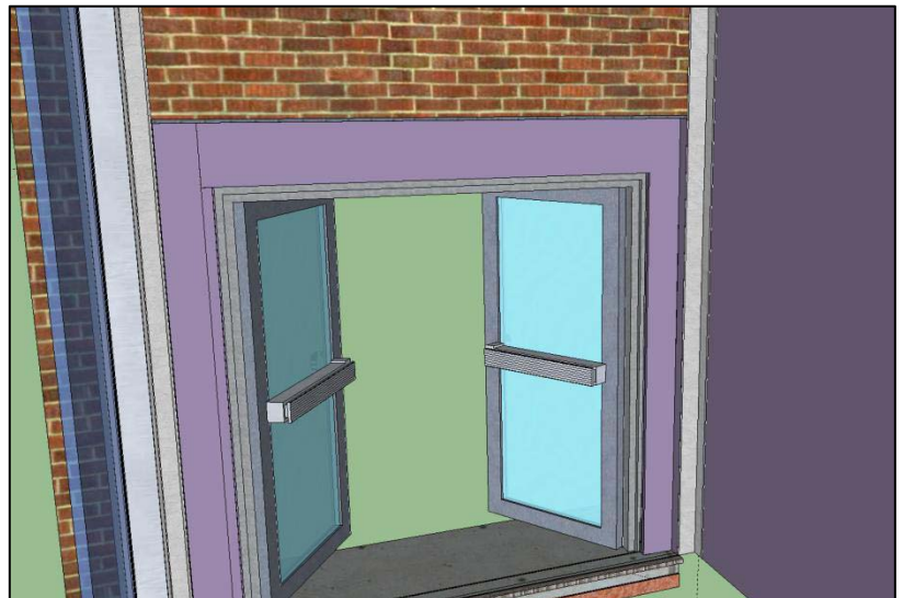
Figure 55 - SketchUp view of the proposed doorframe in place providing a means of egress to and from the existing building. Model created by Chris Pozza.
