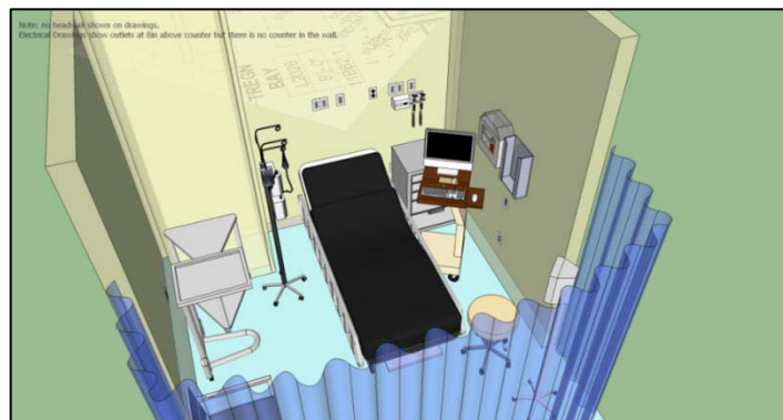
Figure 49 - Mock-up of a patient room for Tyson's Corner. A mistake found here was that electrical drawings specified outlets were to be placed 8" above the counter, but no counter exists in this room. Image courtesy of Shane Goodman.
